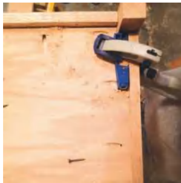
STEP 8. Aligning the corner bolts for the bottom was difficult, so I opted for pocket screws instead
